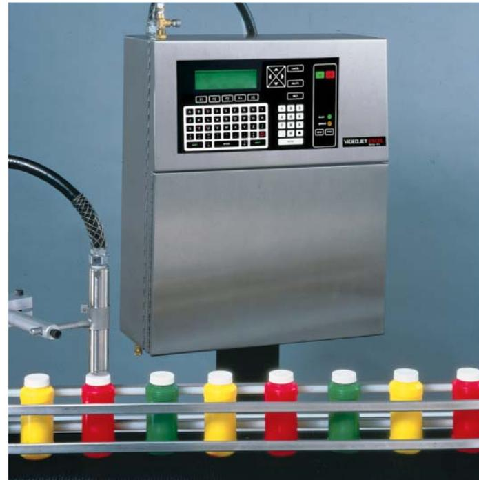
Figure 5 - VideoJET Excel printer in a production line
