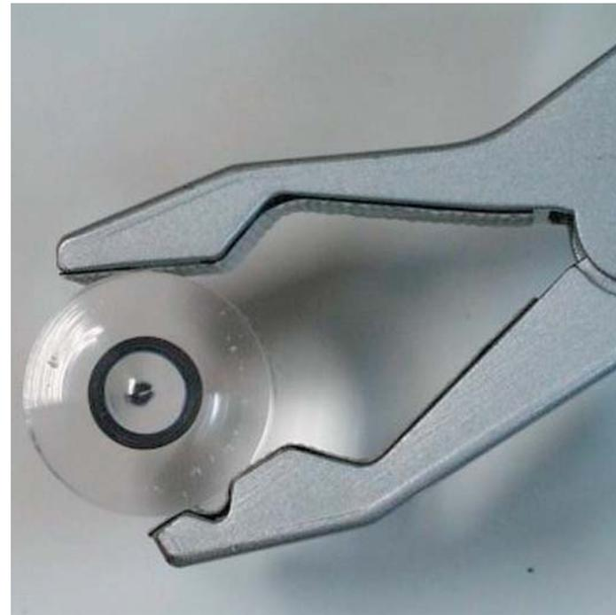
**Figure 2** - An example of an injection-molding product is the laser pick-up for compact disc players. It consists of an aspherical optical lens with a diameter of 4 mm whose conformity to the mold is within 0.1 thousandth of a millimeter. When this component leaves the mold it is ready for final assembly
