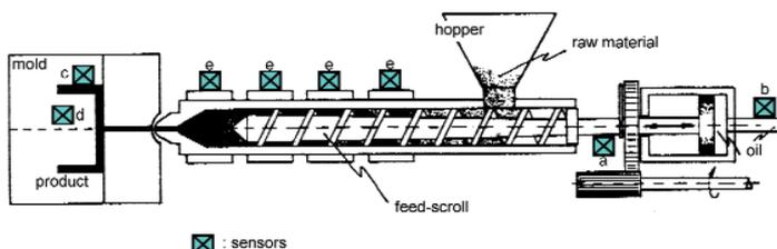
**Figure 1-** A schematic picture of a plastic molding machine. Indicated are the sensors for feed scroll position (a), hydraulic pressure (b), cavity pressure (c), mold temperature (d) and melting temperature (e).
