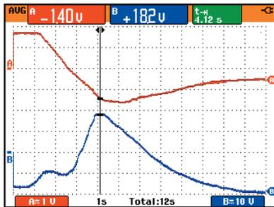
**Figure 3** - The position of the feed-scroll (trace A red) and behavior of the hydraulic pressure (trace B blue) shown as a function of time (Fluke 199C)
