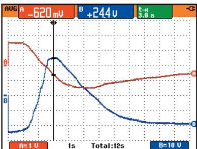
**Figure 4** - The position of the feed-scroll (trace A red) and course of the cavity pressure in the mold (trace B blue) shown as a function of time (Fluke 199C)
