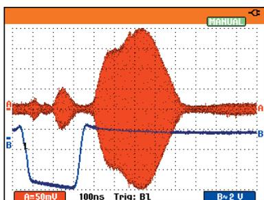
Figure 7: The Fluke 190C is used here with 'Digital Persistence' to capture a natural envelope of a short duration burst of an RF-carrier.
