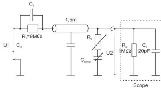
Figure 9: Typical circuit of a 10:1 Scope Probe
