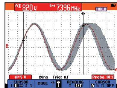
Figure 7: Cursors placed at maximum period, lowest frequency. See actual waveform in red
