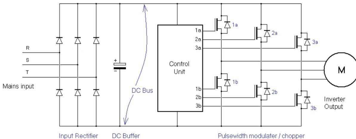
Figure 1: Basic structure of variable-speed drive.
