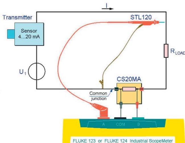
**Figure 6** – Connecting the current sensor CS20MA and a voltage probe to the Fluke 120-series ScopeMeter the proper way, using a common reference junction
