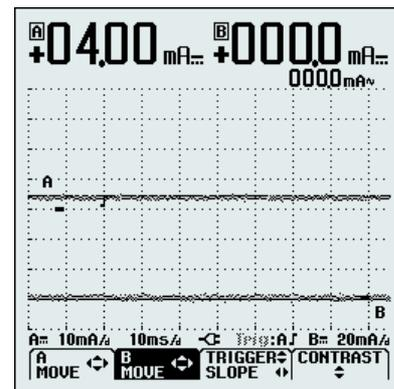
Figure 3 – ScopeMeter measures loop current on two inputs simultaneously, it displays the measured values and gives the oscilloscope display of each current
