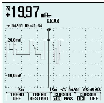
**Figure 4** – TrendPlot makes a graphical recording of the current measurements. Here also an interruption of the current was recorded, indicating a wiring problem
