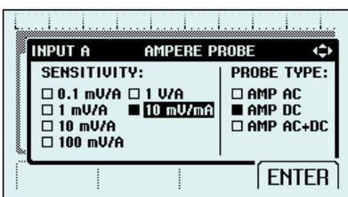
**Figure 5** – When using the CS20MA Current Shunt, the instrument can take the resistance value into account and give the proper current readings automatically
