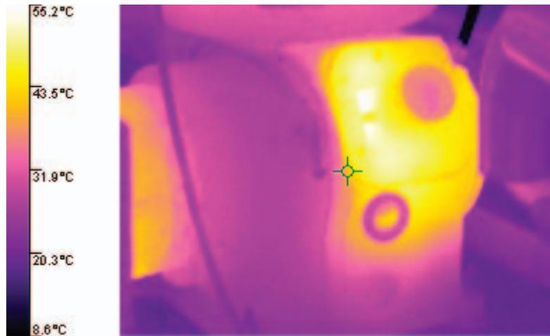
The gearbox of the separator motor, showing extreme (white) hotspots.
