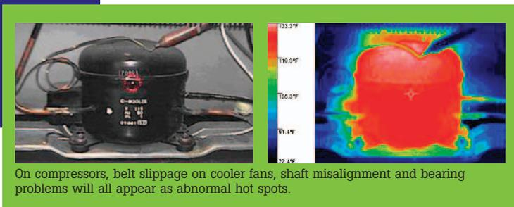
On compressors, belt slippage on cooler fans, shaft misalignment and bearing problems will all appear as abnormal hot spots.
