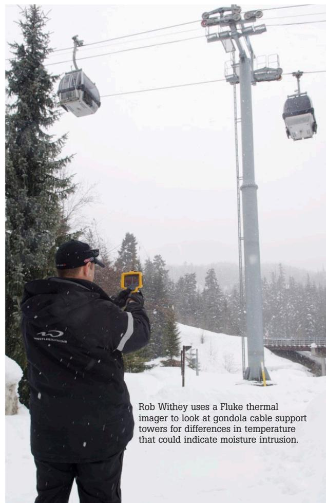
Rob Withey uses a Fluke thermal imager to look at gondola cable support towers for differences in temperature that could indicate moisture intrusion.
